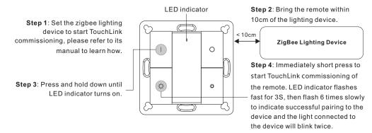
Note: 1) Directly TouchLink (both not added to a ZigBee network), each remote can link with 30 devices.
