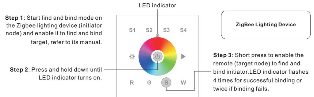
**Note:** Each remote can bind max. 30 lighting devices.
