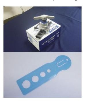
• Manual flaring machine for aluminum pipe for the connection of air conditioner.
